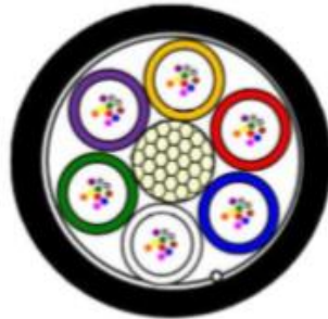
Fiber-optic microcable cross section
